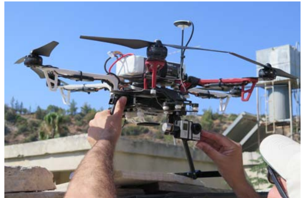
Figure 4. F550 hexacopter with attached GoPro camera
