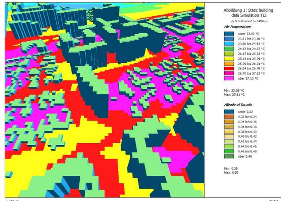
Figure 3. The 3D Air temperatures at the elevation  $z=1.4$  m
