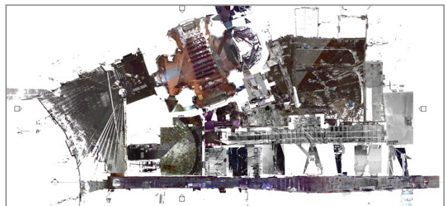
Figure 3. Palazzo Penne, plan view. Pointcloud in Autodesk Revit. Processing: C. Tarantino, M. Pulcran
