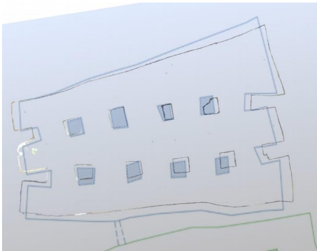
Figure 1: Visual comparison of 2D drawing of the Roman cistern at Eleftherna (light blue; edited from Figure 1 Tsigonaki and Yangaki, 2013, p. 432) and tomography from 3D laser scanning (black line of points; laser scanning section from G. Cantoro).
