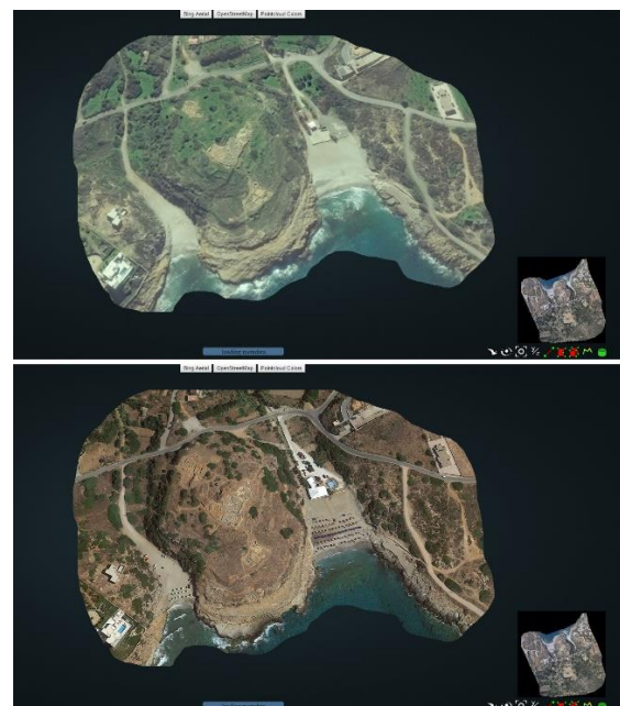
Figure 7: 3D point-cloud with two different colour textures (from original aerial photographs and from Bing provided image), thanks to the combination of Potree and OpenLayers libraries (elaborated on Proof of Concept provided by Potree demo website).
