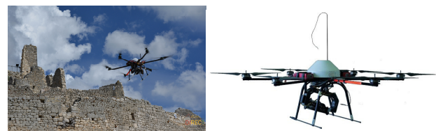
Figure 2. The employed platform - UBIK DIATI MK01
