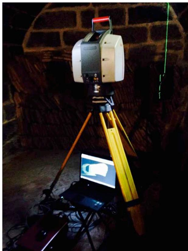
Figure 8. The laser scanner surveying the upper spaces.
