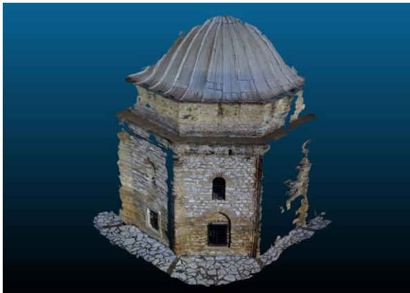
Figure 6. (a) SLAM reconstruction of .svo files in ZED Fu (b) mesh output of one .svo file.
