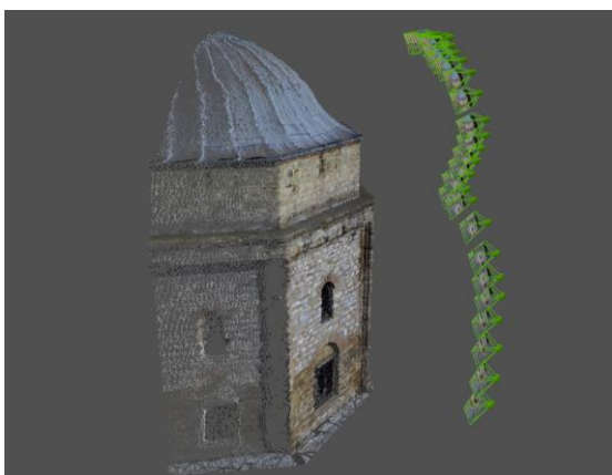
Figure 7: SfM/MVS reconstruction of ZED video frames using Pix4Dmapper Pro.
