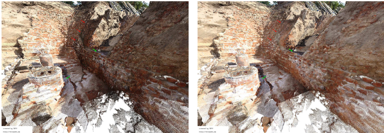
Figure 6. Stephanitorzwingler, Bremen, Germany. Details from the point cloud before (left) and after optimization (right) with equal point density. Note the scattered dark pattern on the brick wall, which disappeared after exposure correction.
