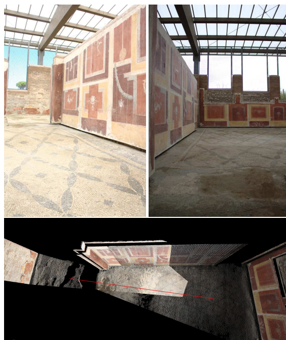
Figure 1. Point cloud of a wall (bottom). The images used for colorization (top) are not radiometrical aligned so the differences in exposure are clearly visible.
