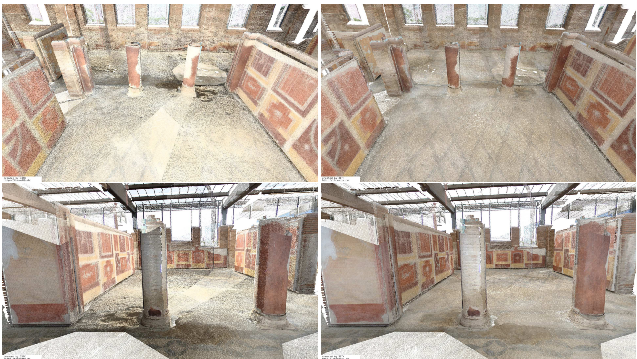
Figure 7. Ostia Antica. Details from point cloud before (left) and after optimization (right). Over- and underexposed images are aligned, therefore the homogeneity in brightness distribution increased. The point density is exactly the same for all images.
