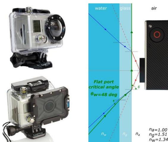
Figure 2. GOPRO HERO dome and flat ports. An early underwater housing with dome port for GOPRO HERO 1 and 2 cameras (left-up). An optional flat port replacement housing for GOPRO HERO 1 and 2 (left-down). A schematic view of the reduced field of view because of flat port critical angle (right).
