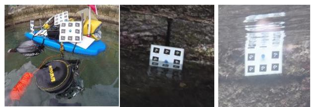
Figure 9. Plates with coded targets used in the experiment.
