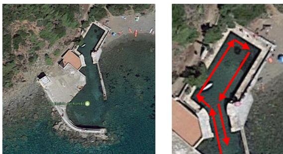
Figure 8. An aerial view of the port structure (left) and an enlarged sight of the rectangular basin chosen for the tests with a schematic view of the photogrammetric strip acquired (right).
