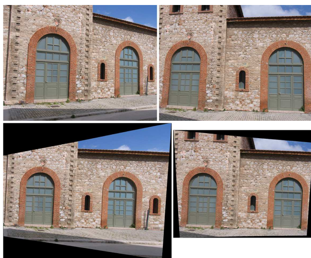
Figure 2. Top row: initial image pair (image axes convergence of 40°). Bottom row: automatically rectified images.
