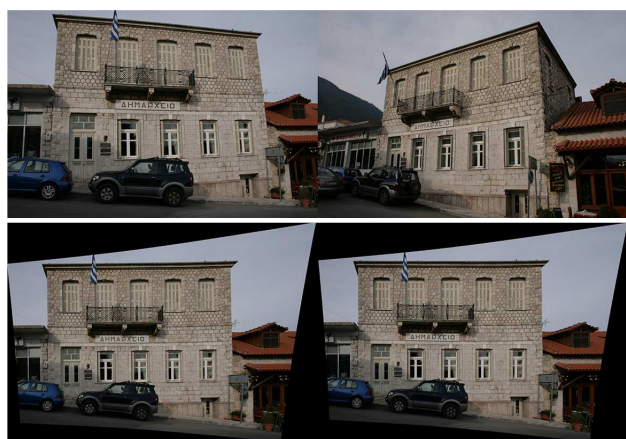
Figure 8. Rectified and rotated left image of the above pair (image axes convergence of 44^\circ ).
