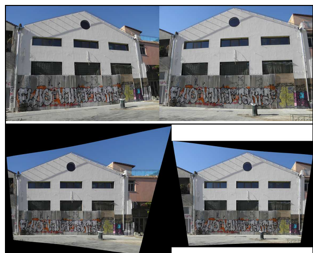
Figure 10. Final rotated images of the above pair (image axes convergence of 25^\circ ).
