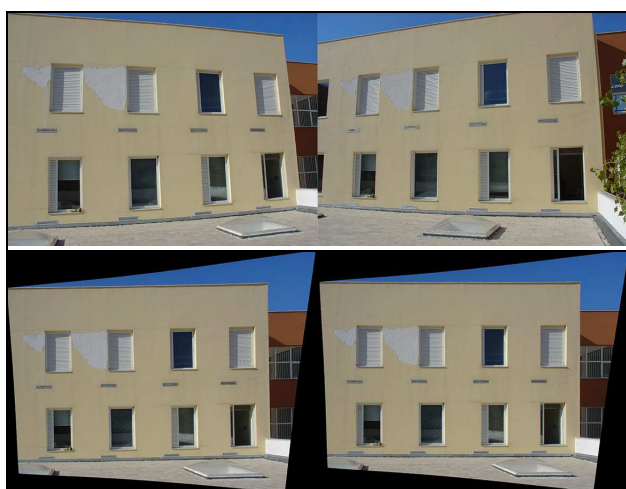
Figure 7. Rectified and rotated left image of the above pair (image axes convergence of 32^\circ ).
