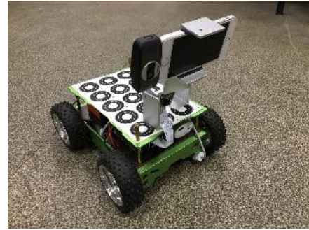
Figure 1. The mobile robot with the FLIR ONE multispectral camera
