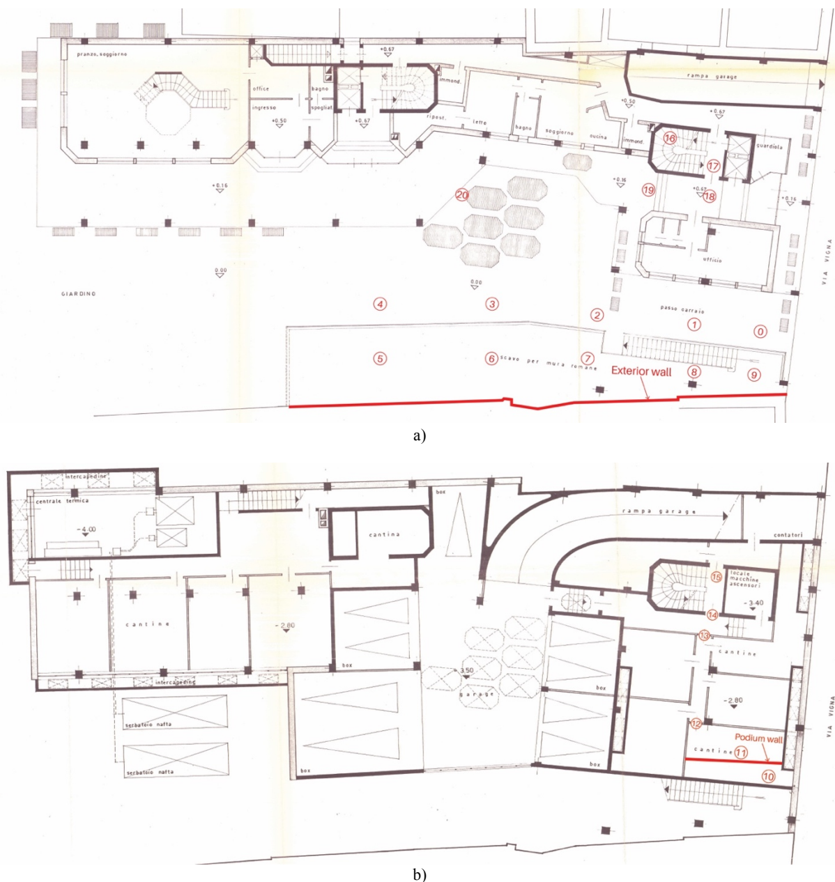
Figure 2. Laser scanner positioning for creating the point cloud represented in Figure 3: a) ground floor; b) basement.
