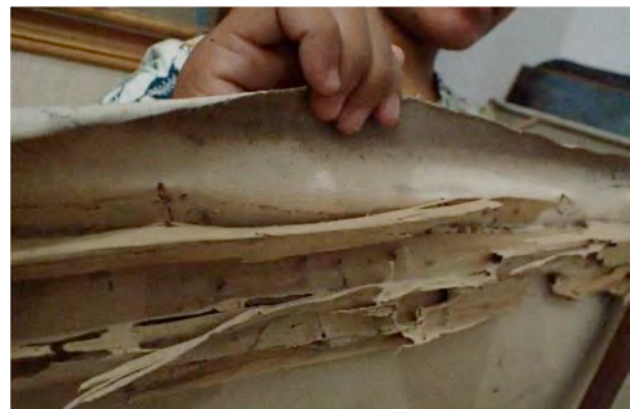
Figure 6: Termite frass in the wooden stretchers (P. Engel 2016)
