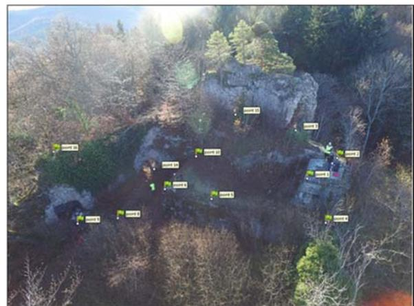
Figure 7: GCPs for model georeferencing.
