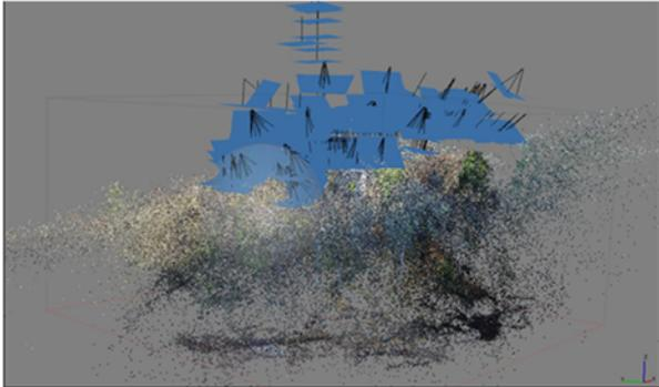
Figure 6: Alignment of pictures taken by UAV (*PhotoScan* software)
