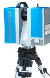
Figure 1. Terrestrial laser scanner(Z+F IMAGER 5010C)
