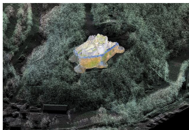
Figure 6. 3D point cloud of the castle of Franchimont combined with the coloured LiDAR data of the municipality of Theux.
