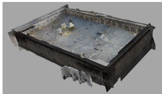
Figure 12. Complex processing of historical photographs to 3D model; inner court is after many attempt still deformed
