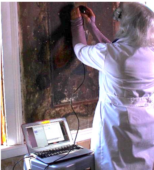
Fig 11: Examination included use of a digital microscope with white, ultraviolet, and infrared light sources. For this conservation project, the Zarbeco MISC_MP2EF-WUVIR was utilized.
