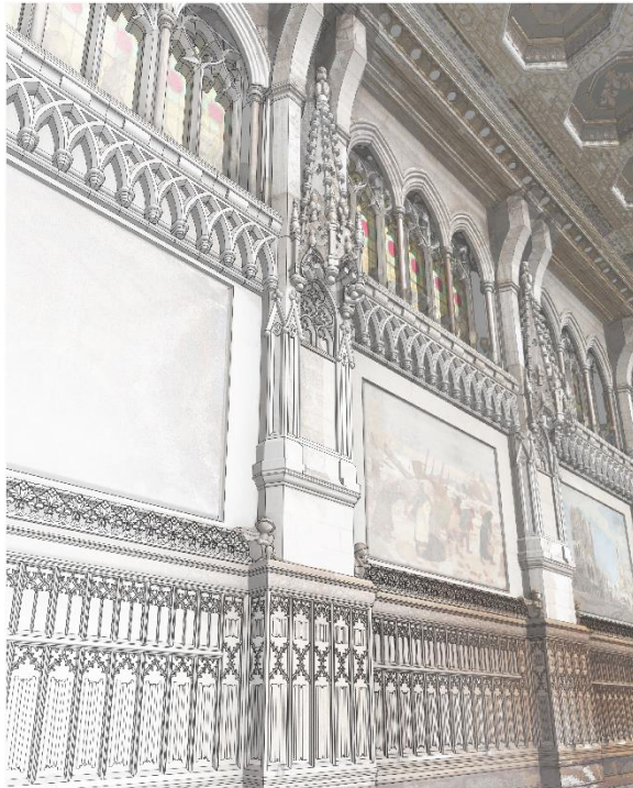
Figure 4: High level of detail BIM overlaid with photogrammetric textured model of the Senate Chamber West Elevation (CIMS, 2017).
