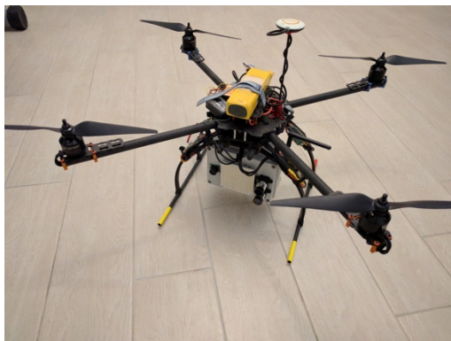
Figure 21 Experimental prototype mounted under a UAV
