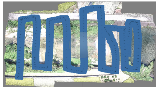
Figure 6. Point cloud data and camera position
