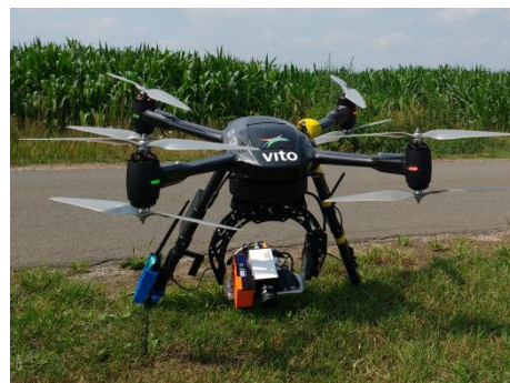
Figure 2. Cubert S 199 ButterflEYE LS mounted on the Aerialtronics Altura Zenith octocopter.
