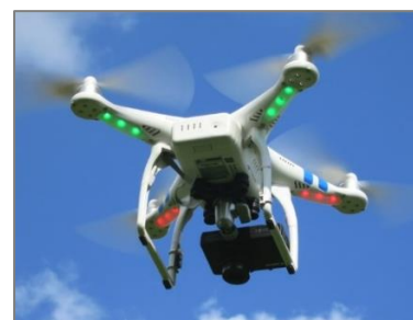
Figure 2. DJI® Phantom 2 equipped with Canon Powershot 110 (Photo G. Bareth, 2014).
