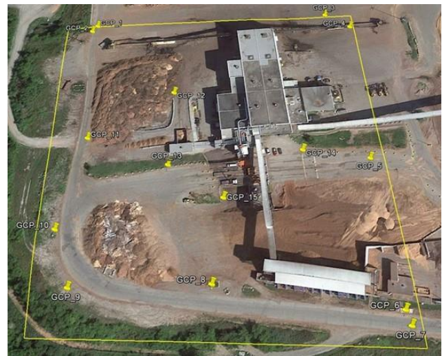
Figure 5: Ground Control Point Layout
