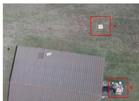
Figure 6. Marker placed on the ground (a) and on a structure in elevation (b).
