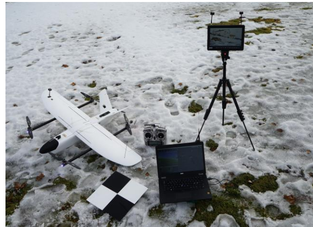
Figure 4. Overview of the equipment with ground station laptop, UAV, ground mark, remote control, and live video screen
