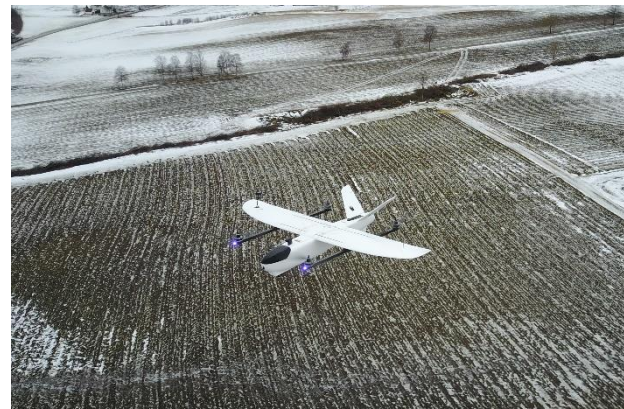
Figure 2. Hybrid UAV with enhanced rotary-wing capabilities, hovering 50 m AGL over the test location at Apelsvoll research station (image taken from a multi-rotor UAV)
