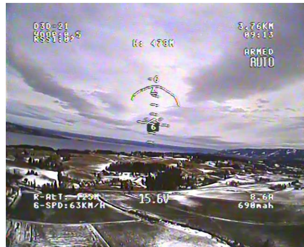
Figure 3. Screenshot of the live video feed of the front camera with overlaid flight data during an autonomous flight over the test area
