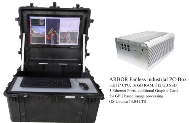
Figure 7: Ground-Station-PCBox (ARBOR FPC-7800-Series)
