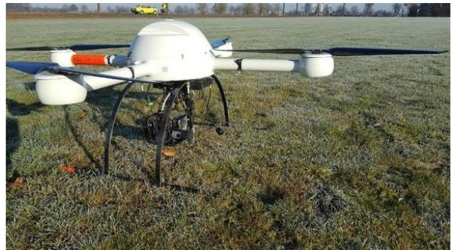
Figure 1. Md4-1000 from microdrones, equipped with thermal and RGB sensors.
