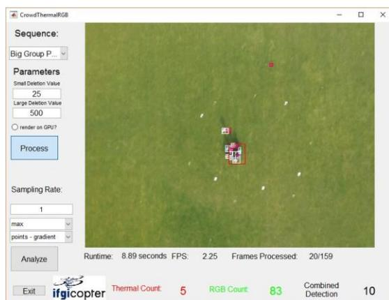
Figure 8. Graphical user interface of the prototype implementation for the combined processing of RGB and thermal video datasets.
