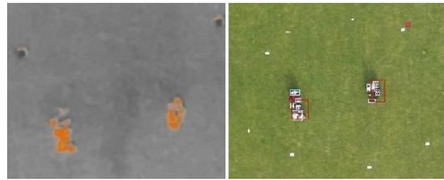
Figure 13. Cropped thermal video frame on the left and the same frame during the processing on the right. The red bounding boxes show detected heat signatures; the white show detected people from the combined approach.
