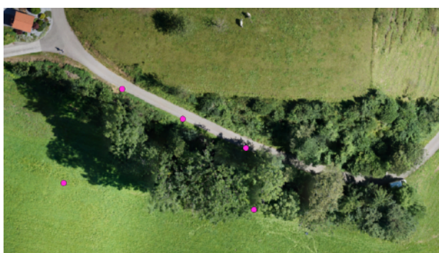
Figure 3. Orthophoto of Test site "Rietholzbach" with ground control points (purple).
