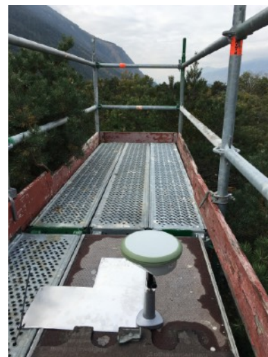
Figure 7. Ground control point with differential GNSS antenna at test site "Pfywald".
