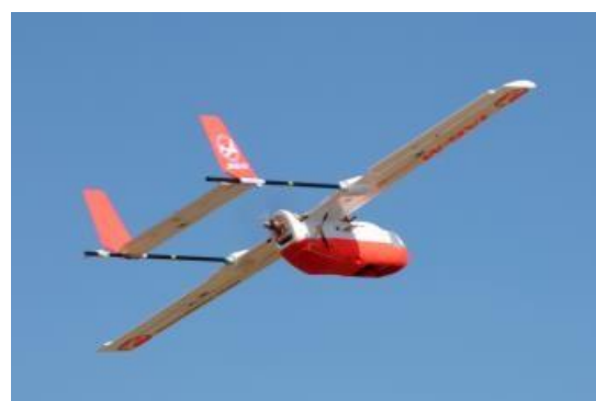
Figure 3. The JAG-M fixed-wing UAV.
