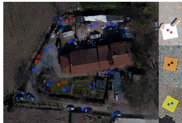
Figure 2. The topographic network (the three vertices in red) and the target measured for the aerial acquisitions (the 12 points in blue). On the right some samples of the employed markers.
