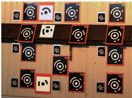
Figure 1b. Different types of coded targets
