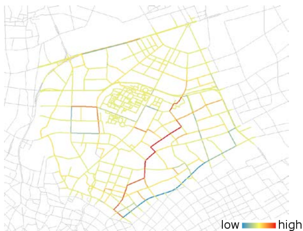
Figure 15. Difference simulated betweenness value between before and after the integration of interior roads into public road network.
