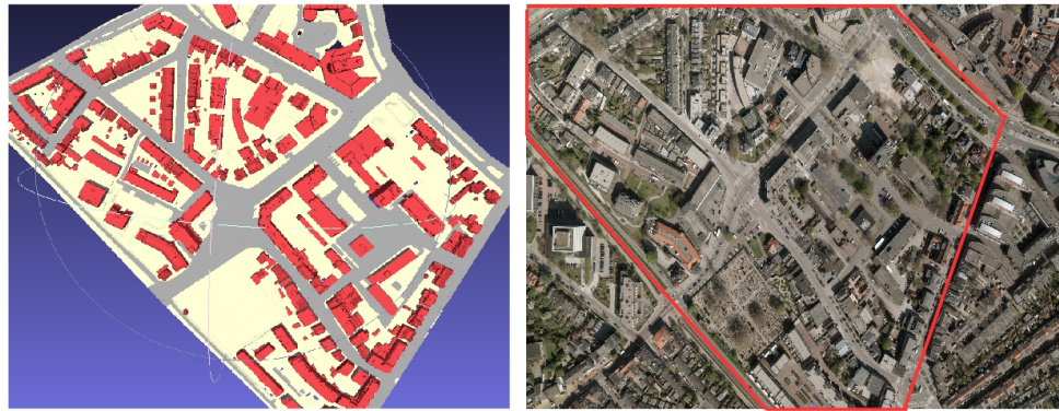
Figure 1. The 3D city models of Amersfoort with 200,000 triangles is created by using a hydrological map and AHN dataset around 2009. The corresponding area of the aerial image in 2010 is shown in the red polygon areas. The different colors in the 3D model show different classes of objects.
