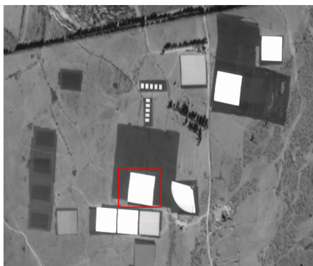
(a) Before correction (with deformed targets in the rectangles)
