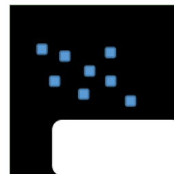
Figure 4. A diagram of fragmentation index calculation Figure 4 shows how to calculate the fragmentation index, domains with an area larger than 1/n of the grid area are represented as white, while domains with an area less than 1/n are represented as blue. It can be seen that number_{total} is 9 and number_{small} is 1, the value fragmentation index is 0.1.
