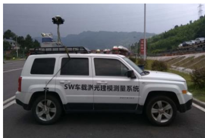
Figure 1. Vehicle-borne Laser Scanning System.
