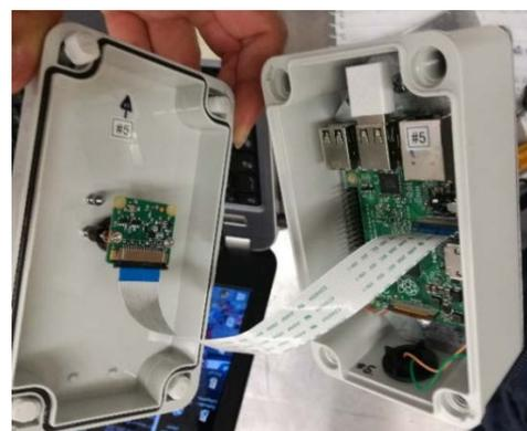
Figure 1. The RPi2B connected with the PiCamera Module V2 in the water proof case designed for the installation of the system in the field.
