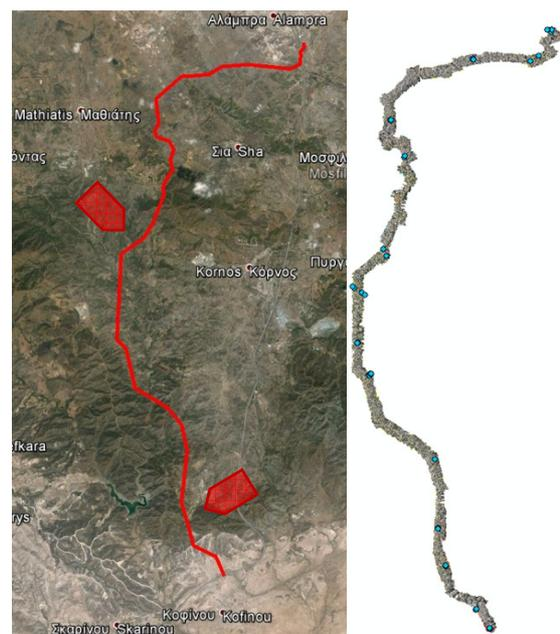
Figure 3. (a) on the left the design of the high voltage line, over google maps, with arrows showing problematic areas, (b) on the right the initial orthophoto using 980 photos and the positions of the 32 used GCPs
