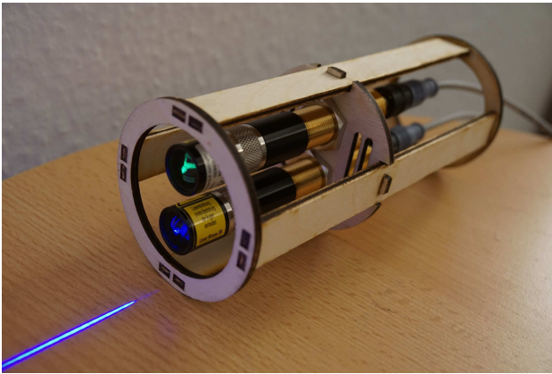
Figure 6: Cross line laser projector in wooden frame employed for the experiments.
