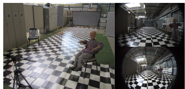
Figure 9. Overview of the experiment (left). Fish eye image (right, bottom) and rectilinear image (right, top).
