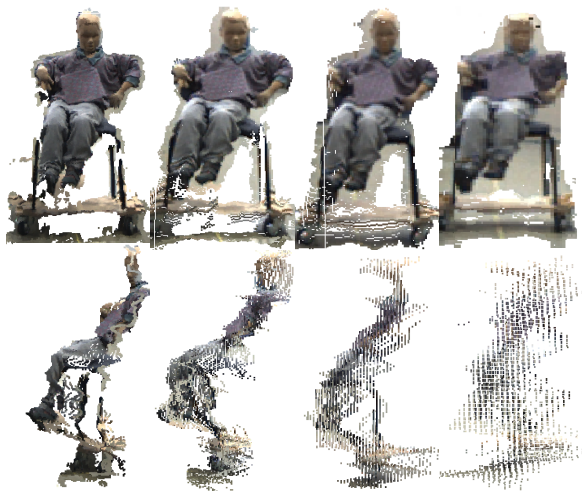
Figure 10. Point clouds for 4,6,8 and 10m distance and 1000lux lighting. The top row depicts four different distances to the camera in a front view. The second row shows the same point cloud from a side view.
