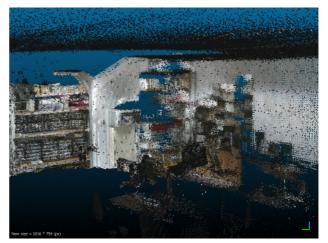
Figure 4. RTABMAP model of our laboratory
