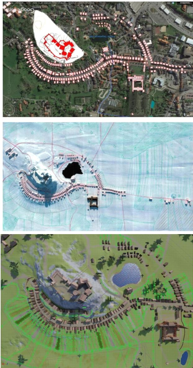
Figure 8. Aerial orthophoto superimposed with historic buildings (top), raw 3D model with landscape and property sketch (centre), and textured 3D model in the Unreal Game Engine (bottom, green lines represent fences for property areas). For better comparison with the engraving, south is up.
