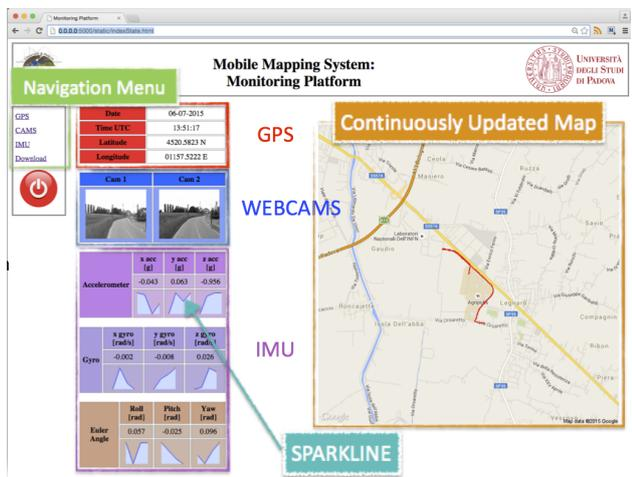
Figure 4. The Homepage of the Mobile Mapping web tool.
