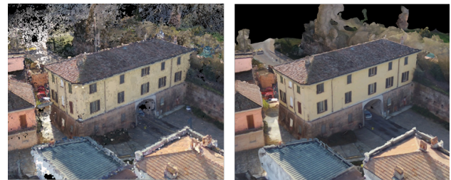
Figure 7. Circular flight, point cloud (left) and mesh (right)
