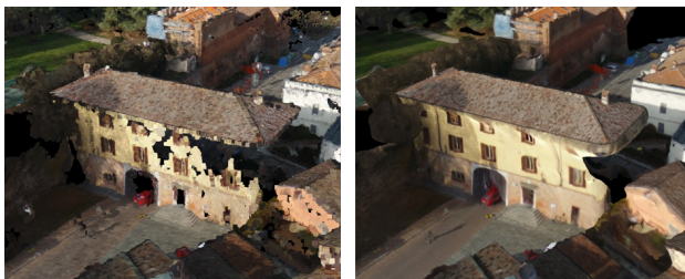
Figure 5. Square flight, point cloud (left) and mesh (right)
