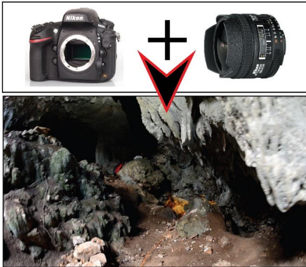
Figure 6. On the top is shown the Nikon D800E and fisheyes lens used: Nikkor 16mm, on the bottom a generic frame recorded during the survey.
