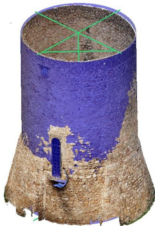
Figure 2. Visualization of the point cloud of the Tower with the standard primitives and the deduction of the central vertex.
