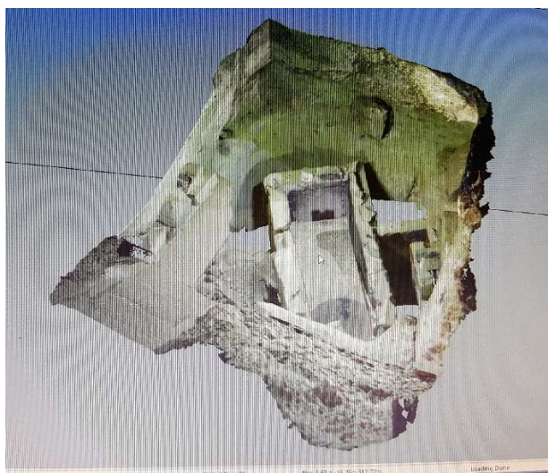
Figure 14. Sarcophagus chamber. 3D model. Scanner Faro focus 3D and SCENE software.
