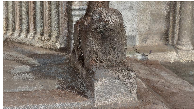
Figure 2: An example of the sparse (left) and dense (right) point cloud produced by jointly processing UAV and terrestrial images featuring different scales, viewpoints, etc. The final dense cloud is noisy and with visible misalignments, due to inaccurate orientation results.
