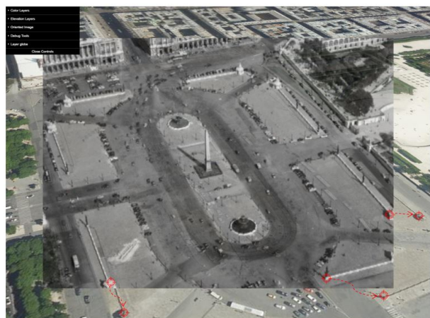
(e) Historical photograph of the place Concorde projected on the DTM in iTowns with the shift highlighted in red.
